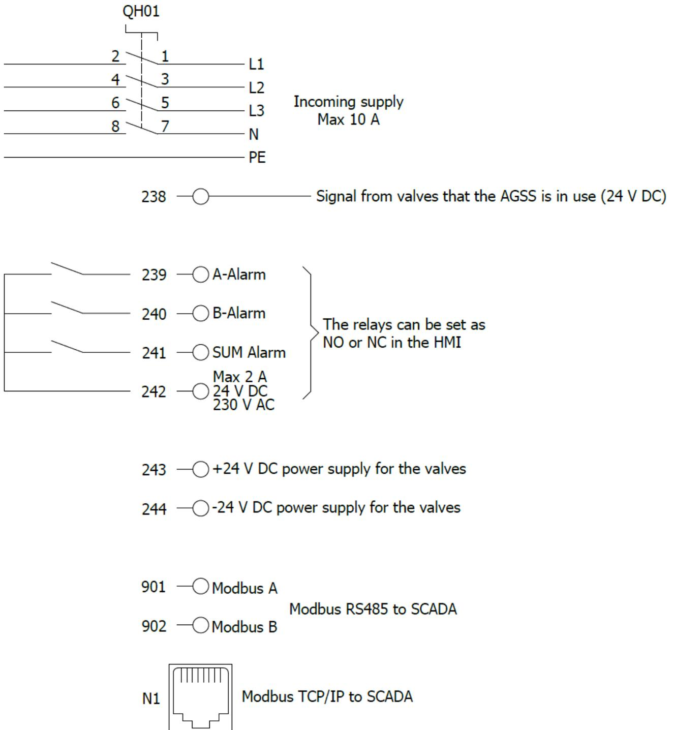
Picture 1 Wiring diagram Power device
