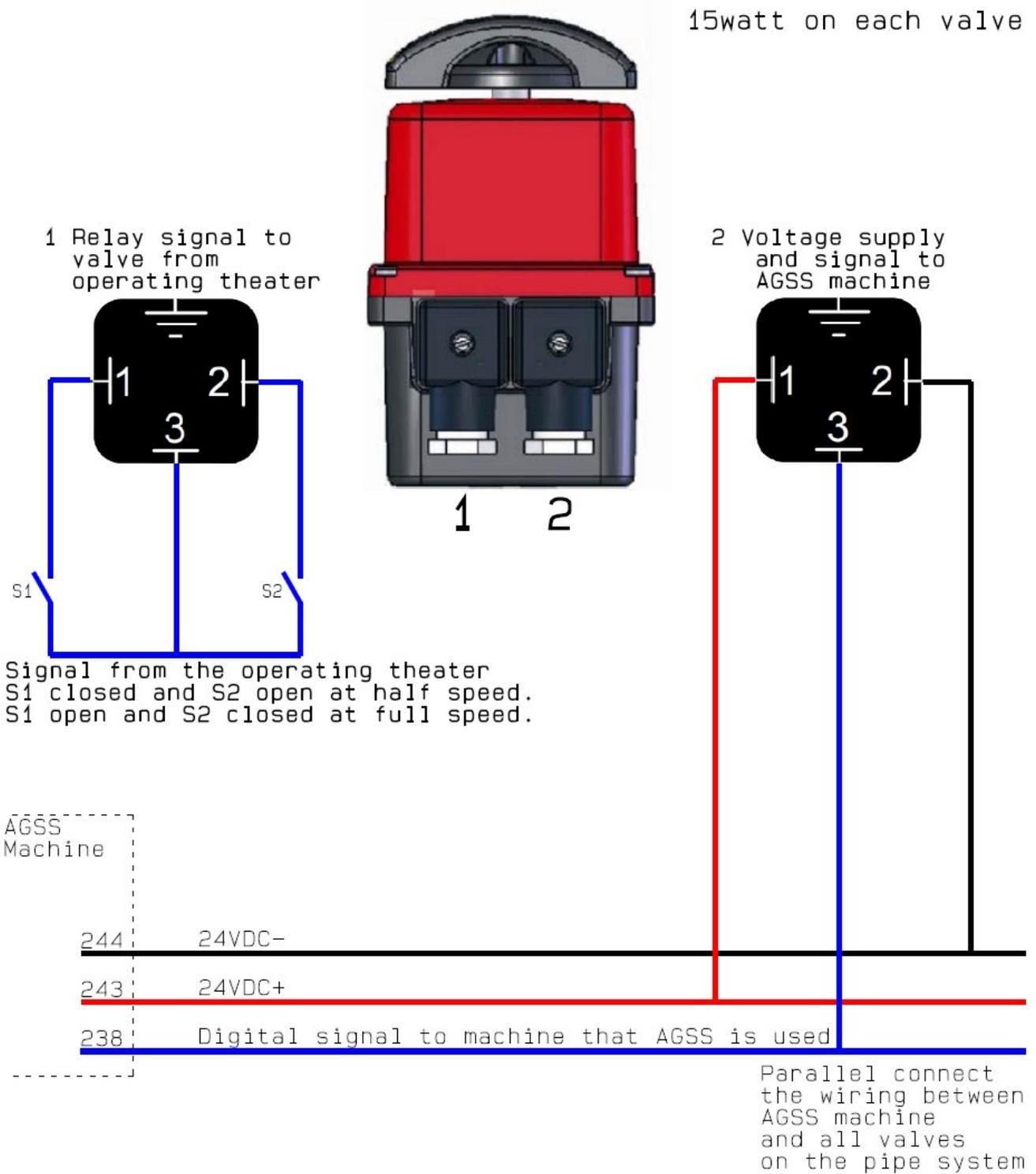
Picture 1 Wiring diagram Regulating valve
