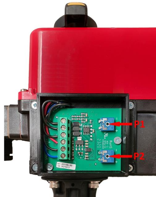
Picture 4 Potentiometer Regulating valve
